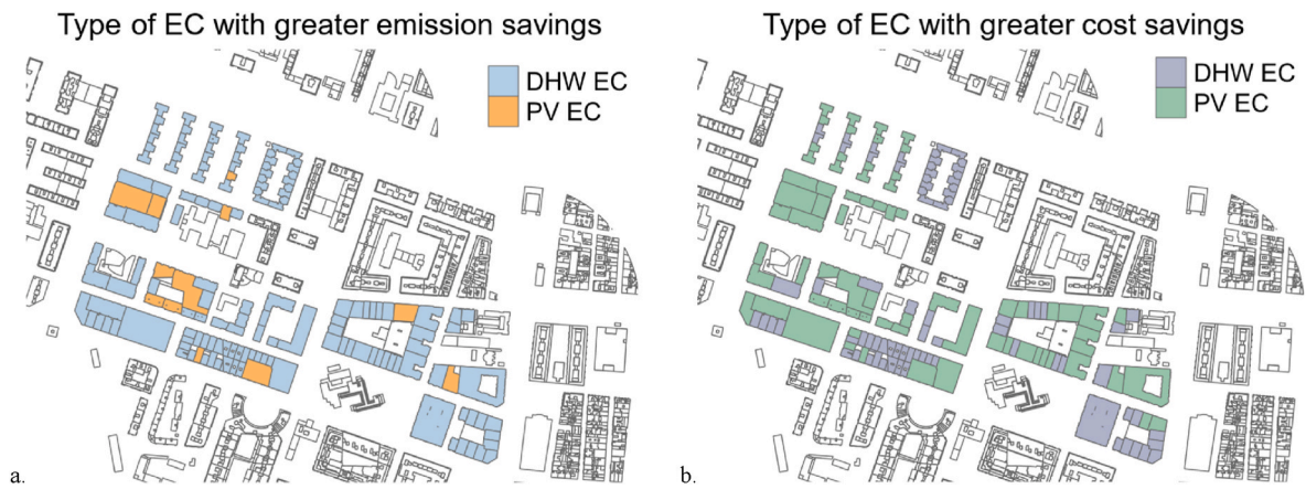
Fig. 10. Identification of best energy efficiency action (DHW EC or PV EC) to obtain. (a) Maximum emission savings and (b) Maximum economic savings.
