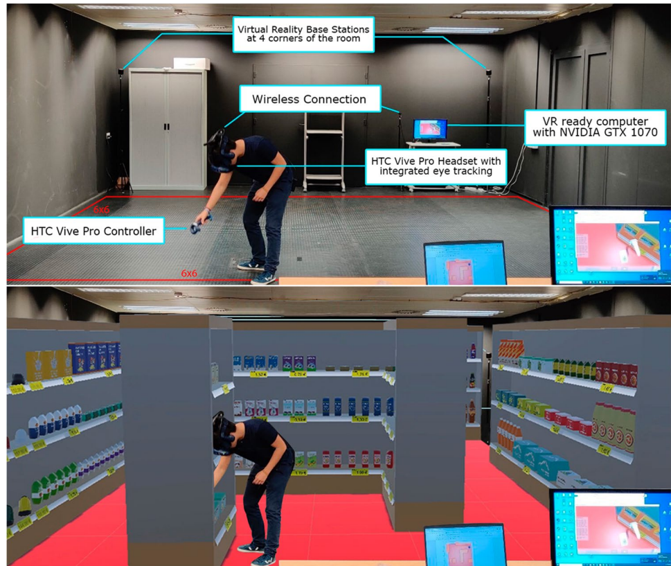
Fig. 1 Above: technology setup employed. Below: VS of 6 m×6 m with seven shelving units and three shelf levels
