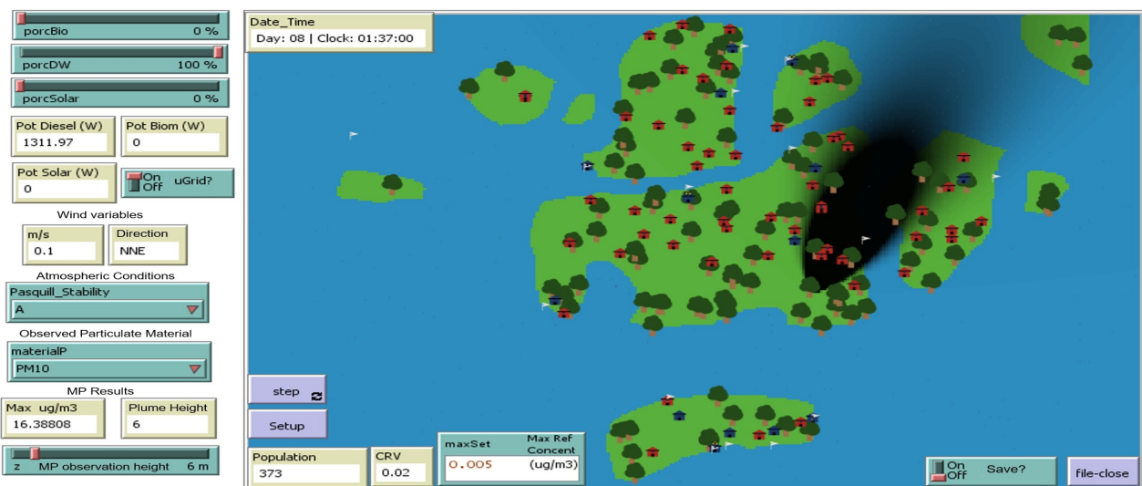
Figure 16. Particulate material dispersion model by Gaussian plume approximation applied in the socio-technological model and implemented in Netlogo. Wind in direction NNE. Atmospheric stability Pasquill A (Unstable). Pollutant PM_{10} .
