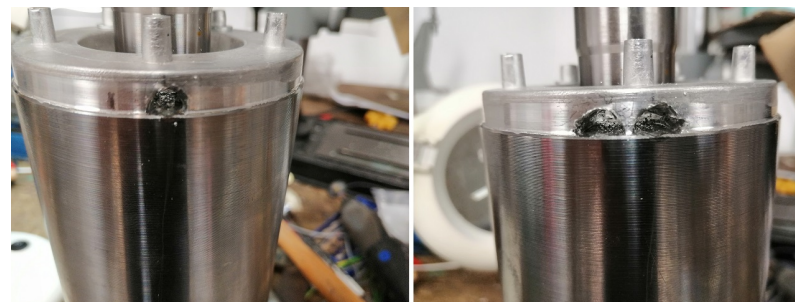
Figure 5. 1 and 2 forced bar breakages.
