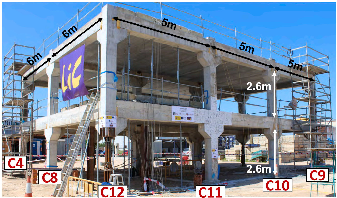
Fig. 1. General overview and dimensions of the building-specimen.
