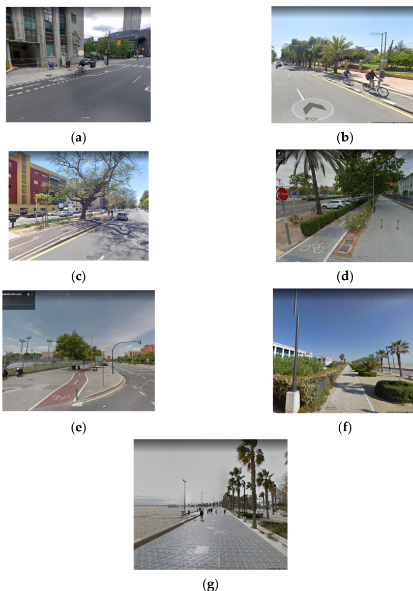
Figure 2. Types of bike lanes: (a) bicycle lane, (b) protected bike lane, (c) sidepath on median, (d) sidepath with vegetated curb, (e) sidepath without curb, (f) bike track, and (g) cycle path [16,17].
