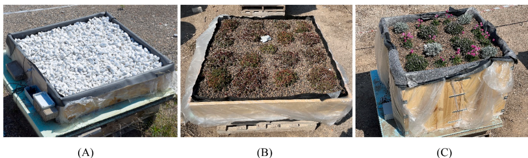
Fig. 2. Scaled model of roofs, at the time of installation (February 25, 2021): (A) traditional with gravel finish; (B) green extensive; (C) green intensive. (For interpretation of the references to colour in this figure legend, the reader is referred to the Web version of this article.)
