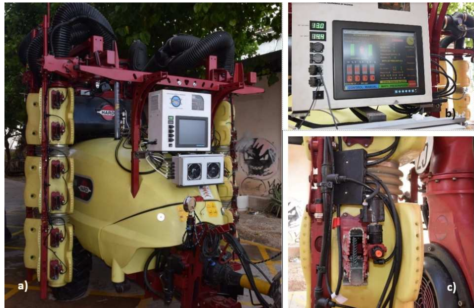
Figure 1. Air-assisted vineyard sprayer with hollow disc-cone nozzles and solenoid PWM valves. (a) General view. (b) Electronic control box. (c) Nozzle-valve assembly.
