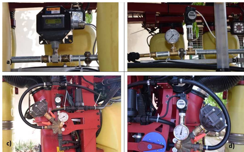
Figure 2. Sensing and measuring system for the modified vineyard sprayer. (a) Flowmeter. (b) Main line pressure sensor. (c) Shock absorber and pressure sensor for leftwing of sprayer. (d) Shock absorber and pressure sensor for right wing of sprayer.
