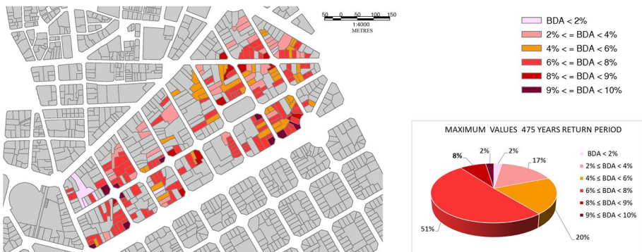
Fig. 30 Built damaged area. 475 years return period maximum values (in %). Façades 480 mm thick
