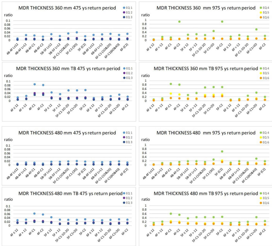
Fig. 25 Mean Damage Ratio (MDR) median values for each constructive assumption and seismic scenario
