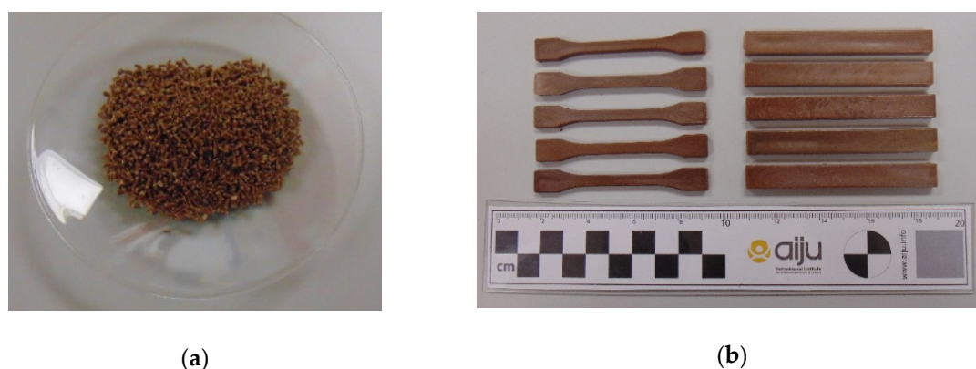
Figure 9. (a) Pellets of Mater-Bi DI01A with 30 wt% almond shell; (b) Injected samples of Mater-Bi DI01A with 30 wt% almond shell.
