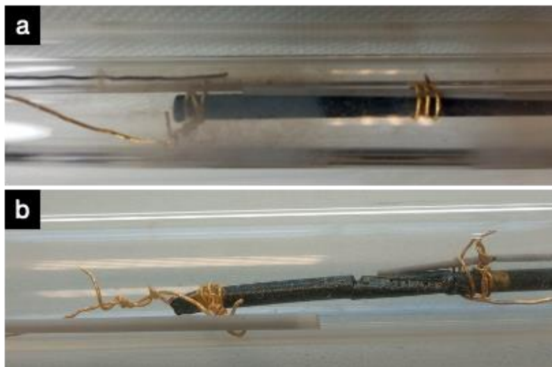
Figure 5. 13. Camera image for the catalytic membrane reactors after ODHE test: a) BSCF catalytic layer; b) CTO catalytic layer.
