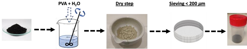
Figure 2. 4. Plastic aid addition in the precursor powder to facilitate the pressing step.
