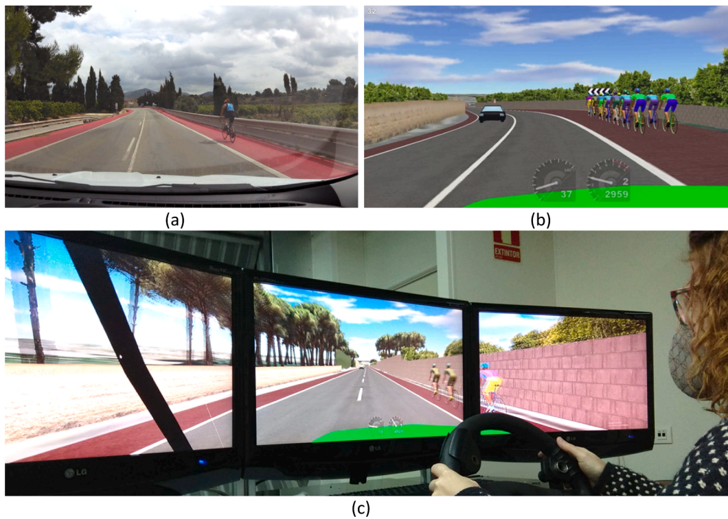
Fig. 3. Images of: (a) real road, (b) road in the driving simulator, and (c) driving simulator test.
