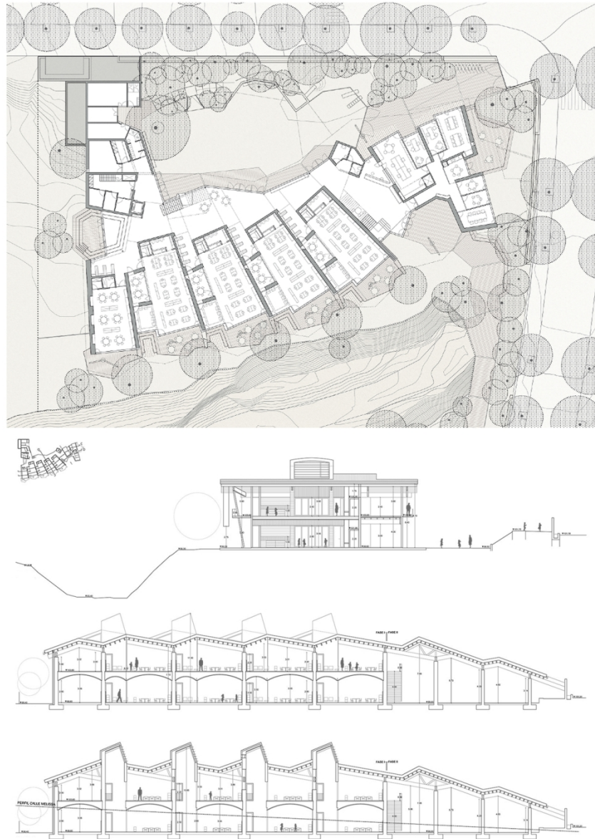
Figure 6: Gradolí & Sanz arquitectes, Imagine Montessori School in Valencia, 2019. Ground plan and cross section. (Credit: Gradolí & Sanz)
