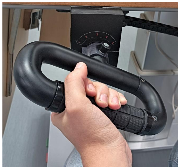
Figure 1. Handle of the measuring device, with marks for 60^\circ (60SUP and 60PRO), 30^\circ (30SUP and 30PRO) and 0^\circ (NEU) postures represented by numbers 1 to 5.
