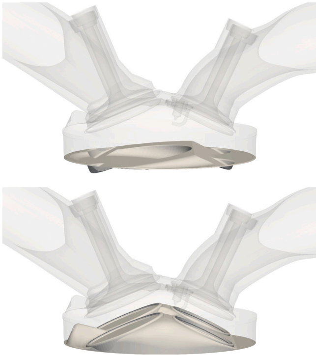
Fig. 13. Baseline (top) and modified (bottom) piston geometries for the compression ratio study.
