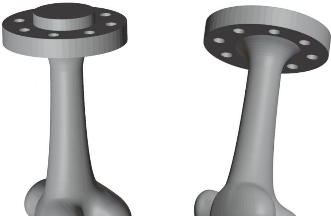
Figure 17. Bones with modified end for attaching to the testing robot
