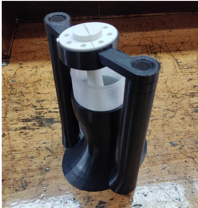
Figure 25. Components of the artificial residual limb assembled in the pouring support before adding the silicone
