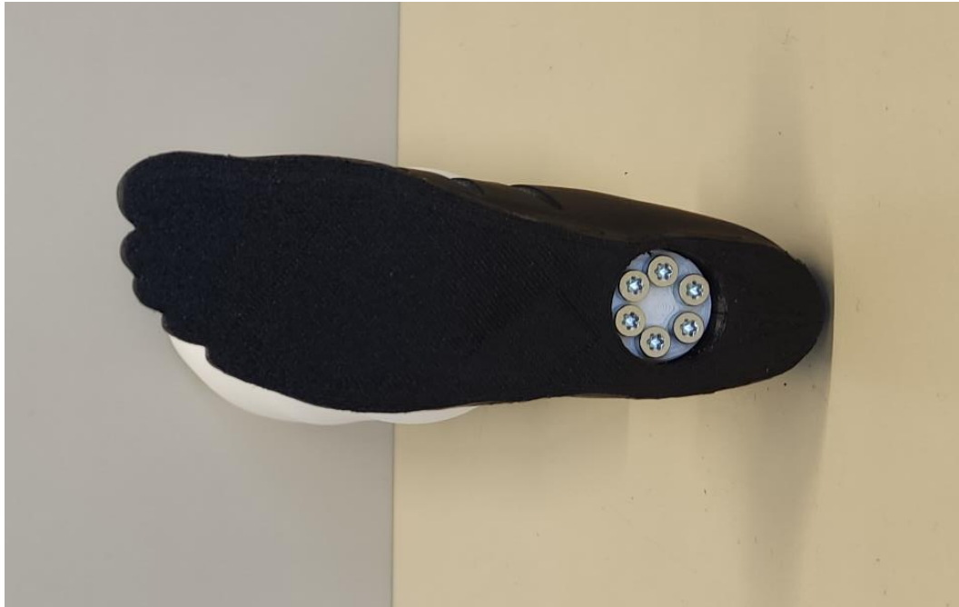
Figure 34. Screws fixing the foot to the pylon
