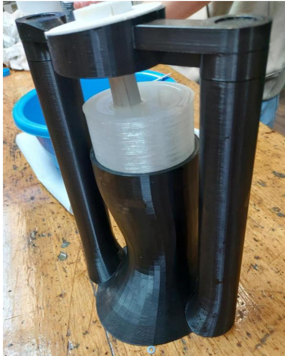
Figure 27. Residual limb with the silicone right after it had been poured
