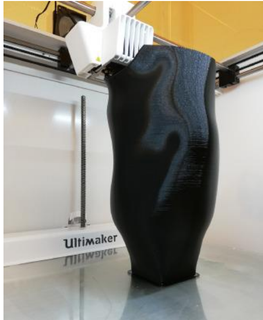
Figure 12. FDM printed lower-limb prosthesis socket [31].
