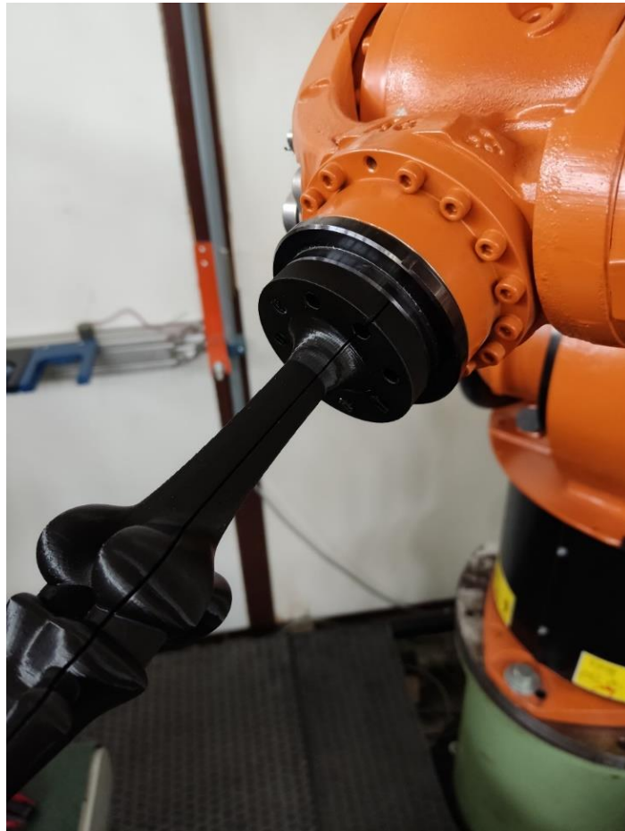
Figure 18. Draft version of the printed bones attached to the robotic arm
