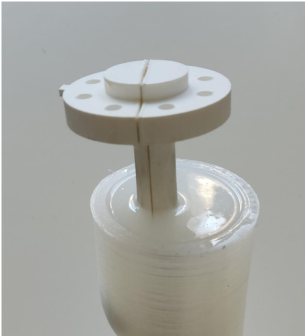
Figure 40. View of the skin filled with the cured silicone
