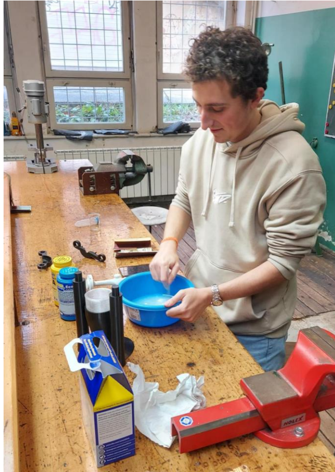
Figure 26. Mixing of both components of the silicone
