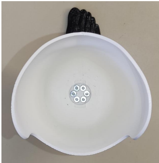
Figure 38. Screws already positioned in the socket to fix the pylon to it
