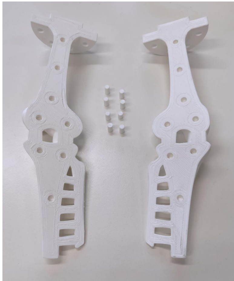
Figure 20. Both separate parts of the printed bones with their pins
