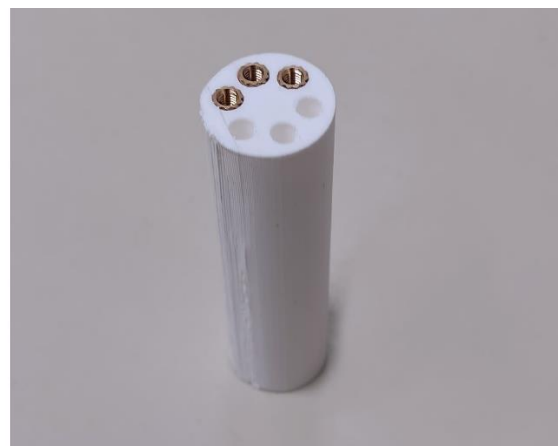
Figure 29. CAD model of the pylon (left) and the printed pylon with three of the six inserts positioned already (right)
