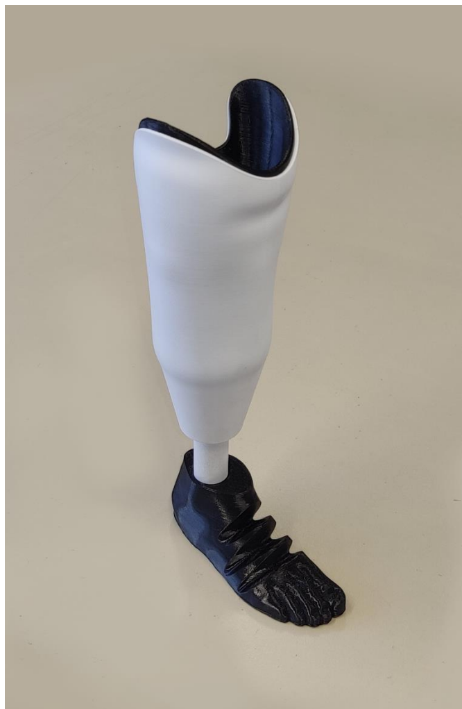
Figure 41. Transtibial prosthetic leg for testing with liner
