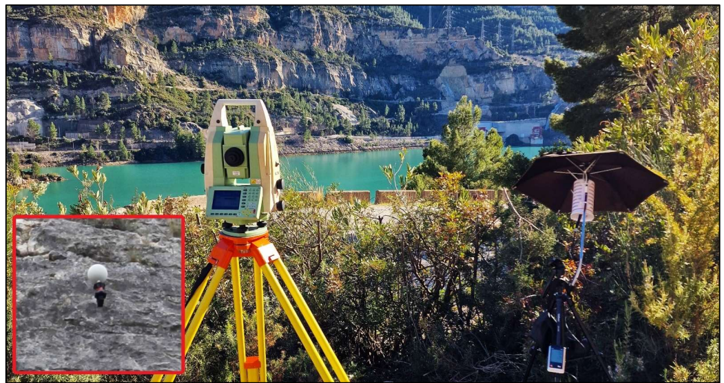
Figure 4. Robotic TS for automatic observation of ChPs during image acquisition. Framed in red is an example of the target installed at the ChPs.
