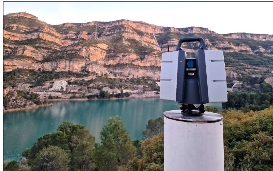
Figure 5. Leica P50 Terrestrial Laser Scanner set up on pillar 8002.
