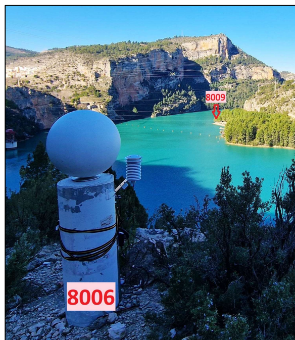
Figure 3. Pillar 8006 is equipped with a \varnothing 0.5 m target sphere and a meteorological data logger used to eliminate the refraction error. Pillar 8009 is marked in red.
