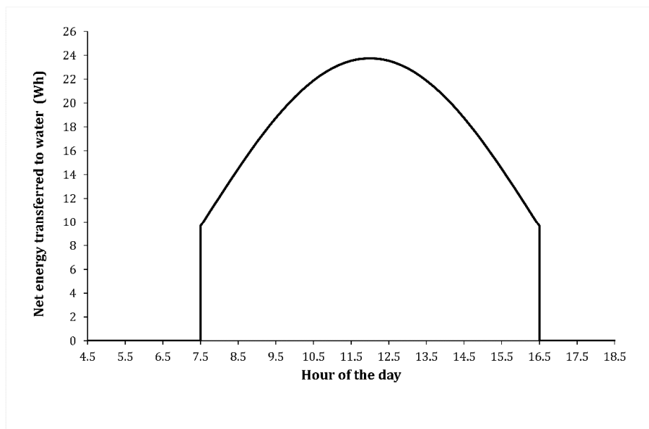
Figure 4. Net power transferred to the water for a single PV panel in the Albamix network.
