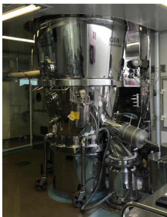
Figure 1. Fluid bed dryer model Fielder Aeromatic MP 6/8.
