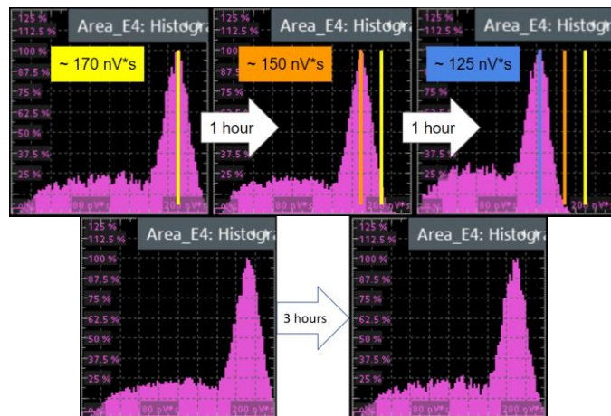
Figure 14. Energy profiles of bBGO pixel. (Top) cFS plots at different time intervals. Glycerin was used at room temperature for this test (25°C). (Bottom) on the left the cFS, on the right the coincidence spectrum after filtering the fast events with rise time below 100 ps. Both using glycerin at temperature below 18°C.
