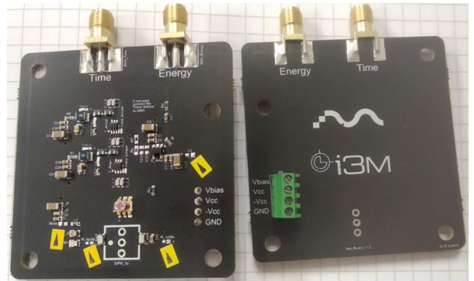
Figure 5. (Top) schematics of the HF-amplifier readout electronics employing a timing amplification stage (TAS) composed of HMC311SC700 bipolar monolithic microwave integrated circuit (MMIC) amplifiers and a wideband Bias-T. (Right) a screenshot of the low noise from the timing signal. The RMS is calculated to be around 330 μV with a small offset of 100 μV. (Bottom) front-end boards, left front-side, right back-side.
