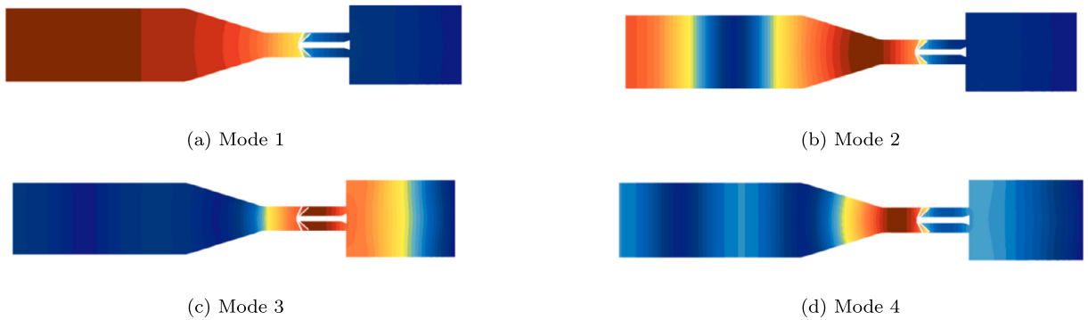
Fig. 14. First four acoustic mode shapes of the EM2C burner.
