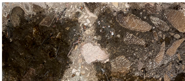
Fig. 8. Effect of ITZ on chloride penetration of conventional concrete specimen.
