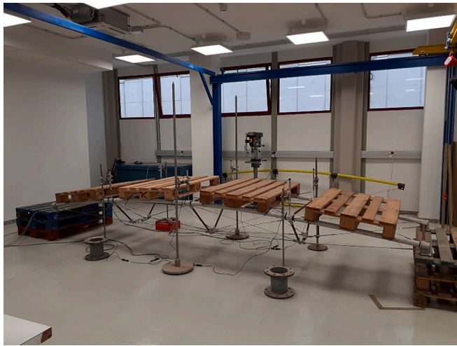
Fig. 8. Small-scale GFRP footbridge prototype using the bending-active bow-string concept [23].
