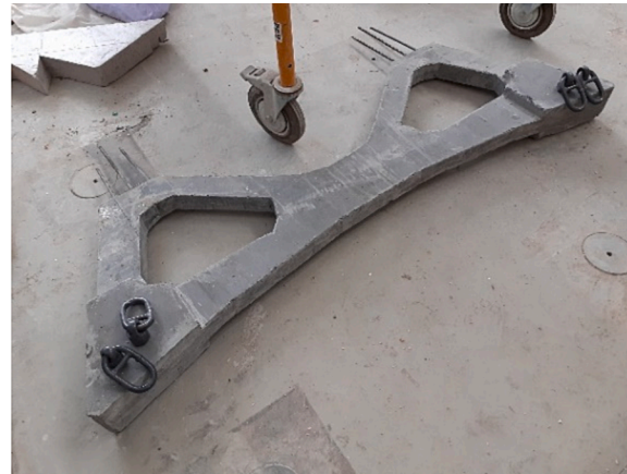
Fig. 16. Casting of the deviator. Left: formwork and minimum reinforcement; right: the deviator after unmoulding.
