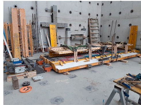
Fig. 16. Casting of the deviator. Left: formwork and minimum reinforcement; right: the deviator after unmoulding.
