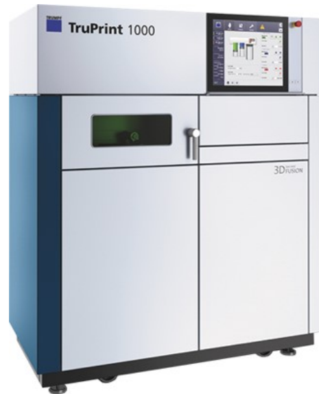
Figure 2.2: TruPrint 1000 L-PBF machine used in this research.
