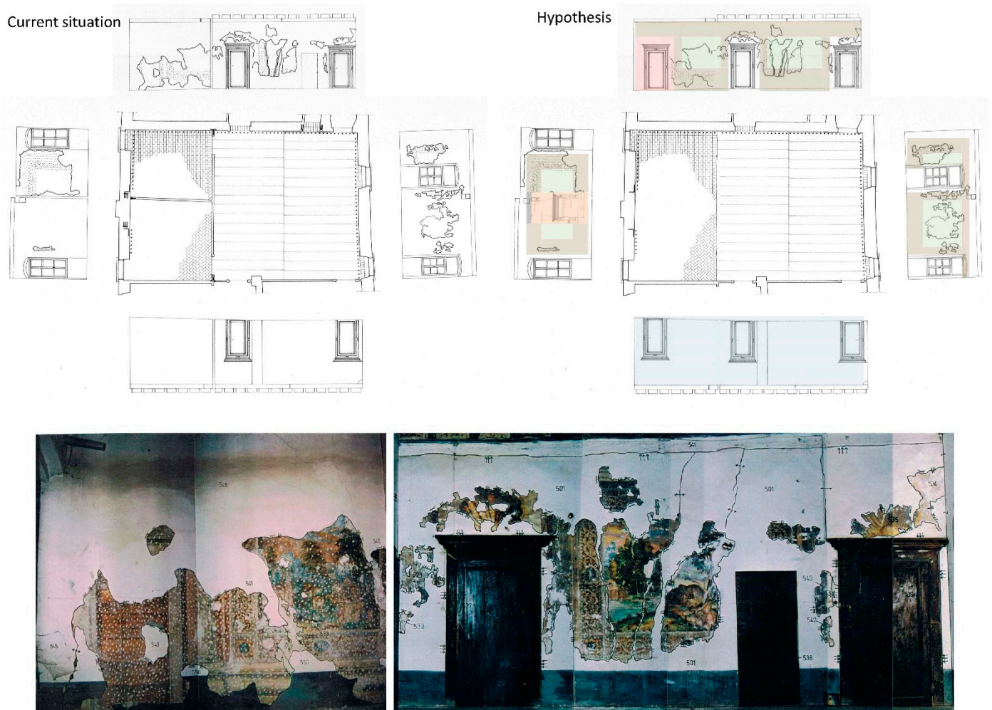
Figure 21. Hypothesis for the reconstruction of the central hall on the first floor.
