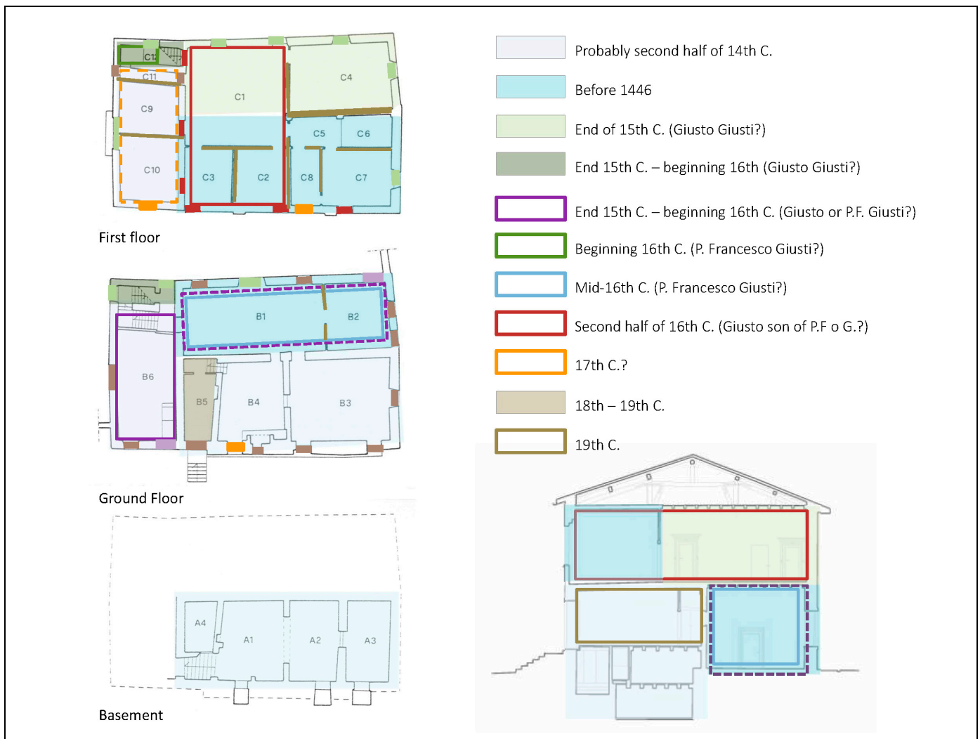
Figure 23. Hypothesis for the phases of construction and transformation of the stately palace of Villa Giusti-Puttini (the letters correspond to the different rooms of the palace).
