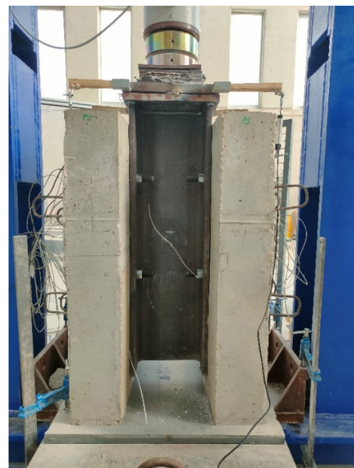
Figure 5 Test specimen at ambient temperature located under the hydraulic jack before being loaded.
