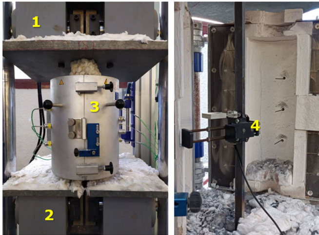
Figure 1 Experimental setup. 1: Upper block. 2: Lower block. 3: Electric furnace. 4: Extensometer.
