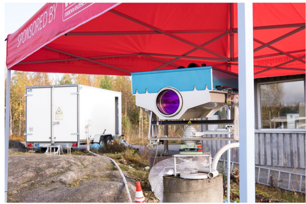
Fig. 3 Multi-wavelength interferometer TeleYAG-II mounted on a pillar in the Metsähovi network. The trailer in the background hosts the optical source and the detection electronics. Trailer and optical head are connected by optical fibres
