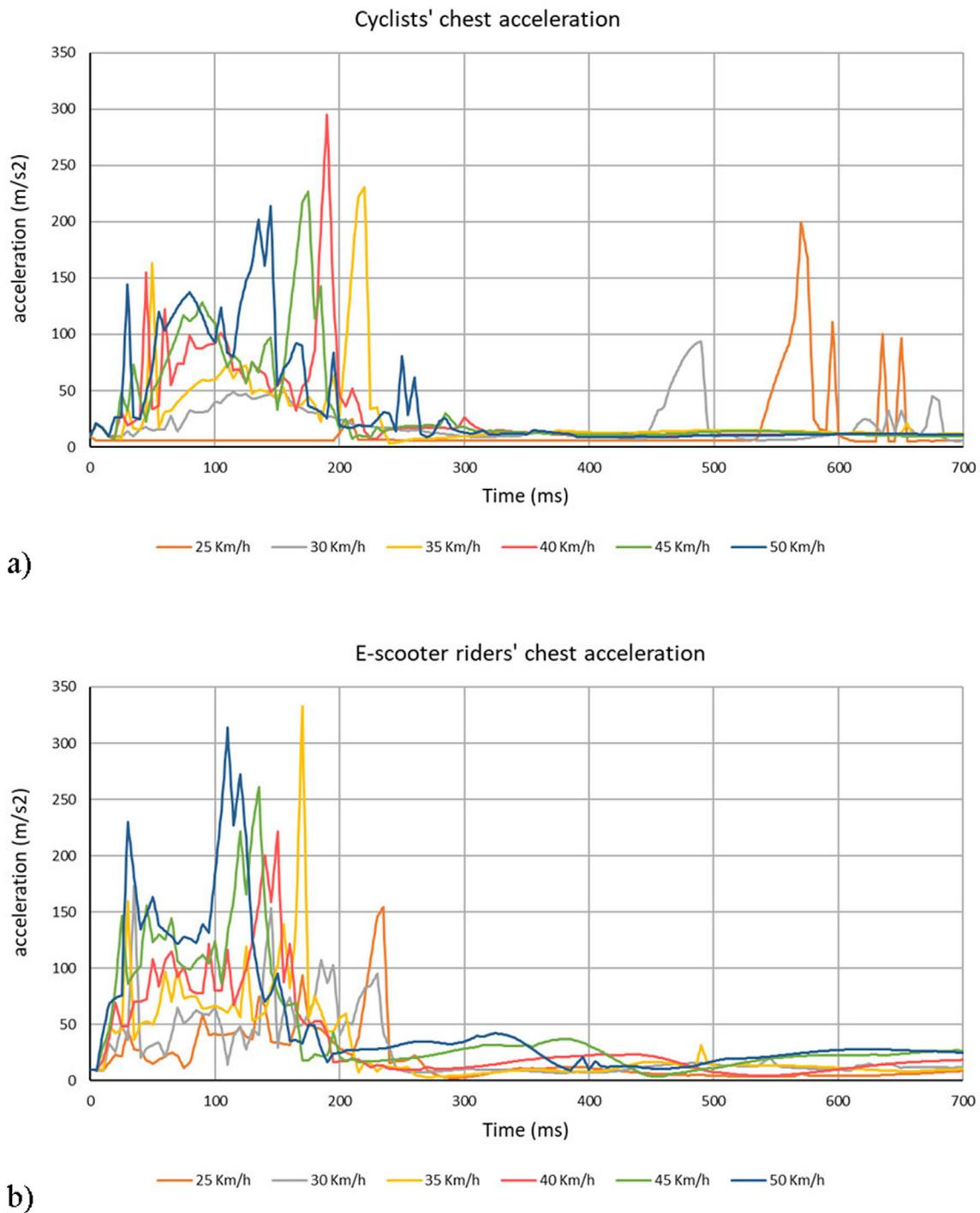
Fig. 6. A) cyclists' chest acceleration, b) e-scooter riders' chest acceleration.
