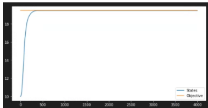
Figure 4.4: Air gap at each time step during 5 seconds, take off from the ceiling
