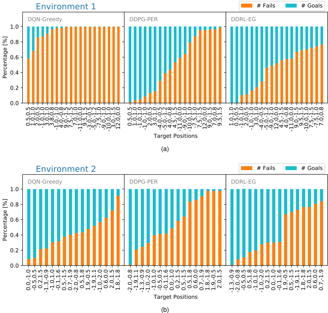
Fig. 12. Each subfigure shows the percentage of success vs. collisions of the agent during the training process of each of the algorithms. (a) DQN-Greedy, DDPG-PER, DDRL-EG. (b) DQN-Greedy, DDPG-PER, DDRL-EG.
