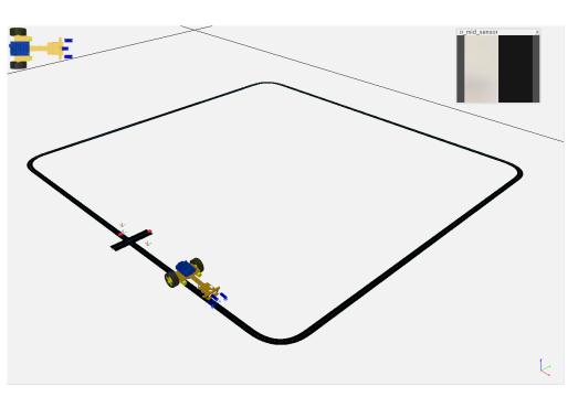
Figure 2. Line tracker in CoppeliaSim robot simulator.
