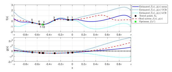
**Figure 1.** Estimated cost function  $\hat{f}(x)$  and safety function  $\hat{g}(x)$  (in solid blue, representing the mean) and real cost and safety functions (in dashed red). The estimated cost function's upper and lower confidence bounds are shown in dotted light blue/cyan colors. The black squares are the tested values  $x_k$ , and the green bullet is the safe minimum value of the estimated cost function. The dashed-dotted black line highlights the zero threshold of the safety constraint.
