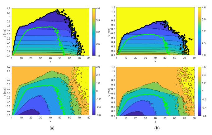
**Figure 5.** Cost function f(x) and safety function g(x): (a) training circuit and (b) testing circuit. The green lines determine the safety limits of each circuit (it is a threshold of g, but it has been overlayed onto f to highlight the admissible search region. The top row shows the plots for f, while the bottom row shows the plots for g.
