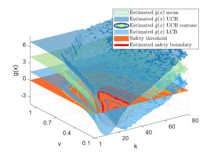
**Figure 7.** Estimate of the safety constraint  $\hat{g}(x)$  from experimental samples at the last iteration: the mean of the constraint is depicted with a green mesh, UCB and LCB are depicted with blue meshes, the orange plane depicts the zero threshold level, and the red contour line determines the estimated safety boundary (other contour lines of the UCB are also shown).
