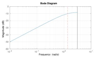
Figure 3. Bode magnitude plot of the control-effort high-pass weight for safety constraint evaluation.
