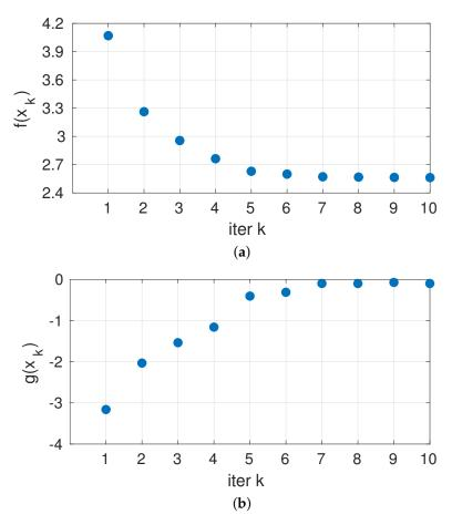
Figure 6. Values of (a) Cost function and (b) Safety function against test iterations.
