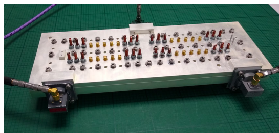
FIGURE 36. Assembled reconfigurable diplexer.
