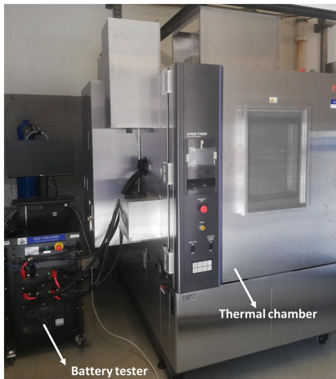
Fig. 1. Test bench for battery cell characterization.
