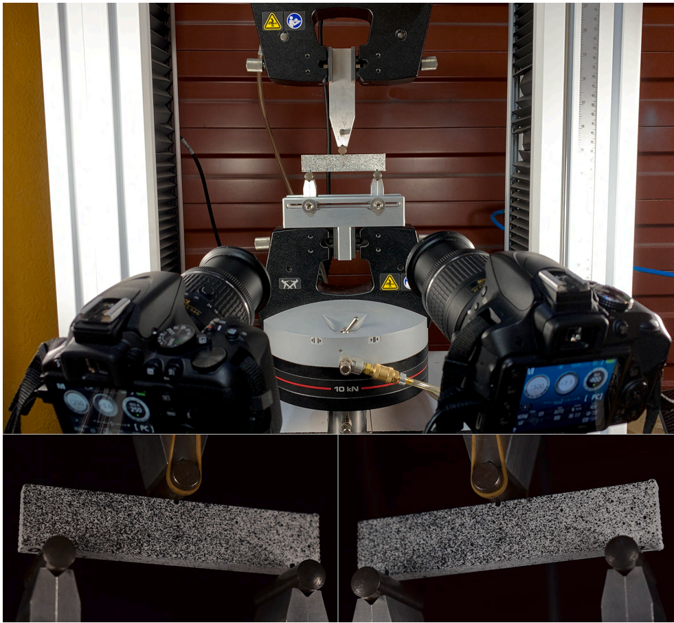
Fig. 6. Experimental setup of the 3P bending test for prismatic specimens with DIC instrumentation (top) and captures from each camera (bottom).
