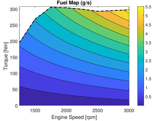
Fig. 1. Fuel map as a function of Torque and Engine Speed acquired from experimental data.
