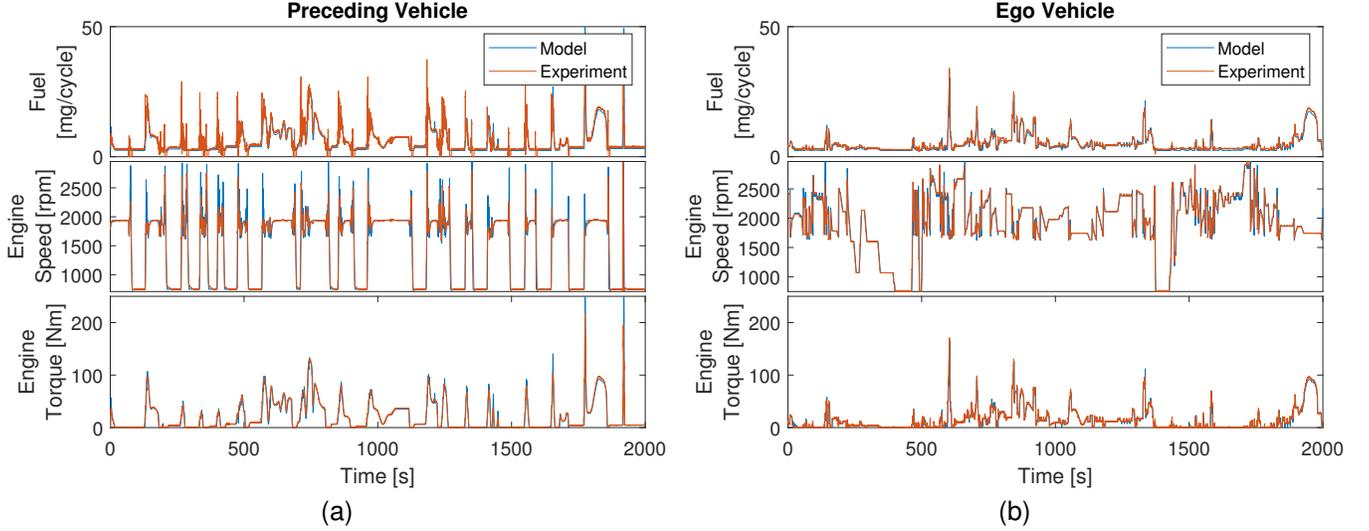
Fig. 6. Comparison of engine torque, engine speed and instantaneous fuel consumption between model and experiment for (a) Preceding vehicle. (b) Ego vehicle.
