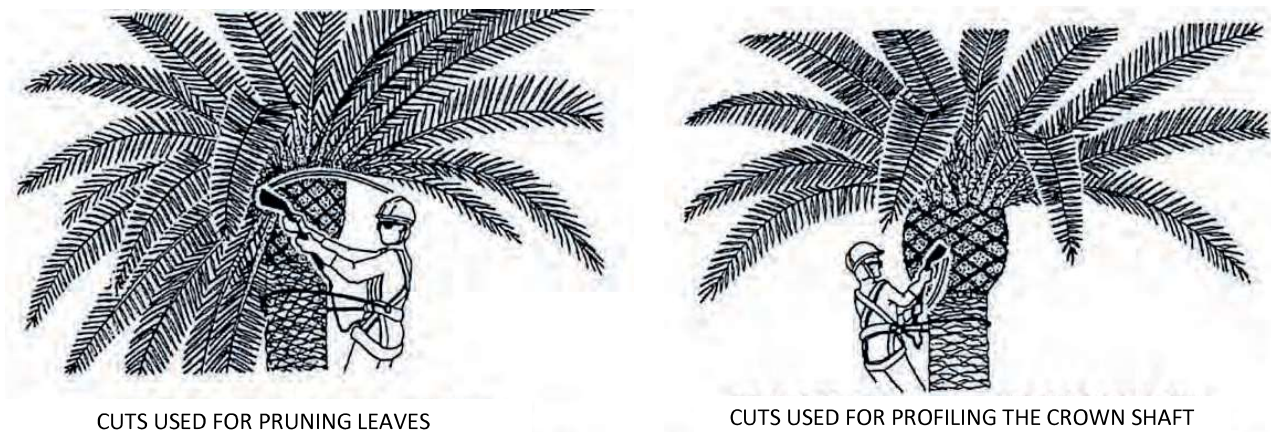
Figure 4.4.1 Different types of cuts. (NTJ 07P COITAPAC)
