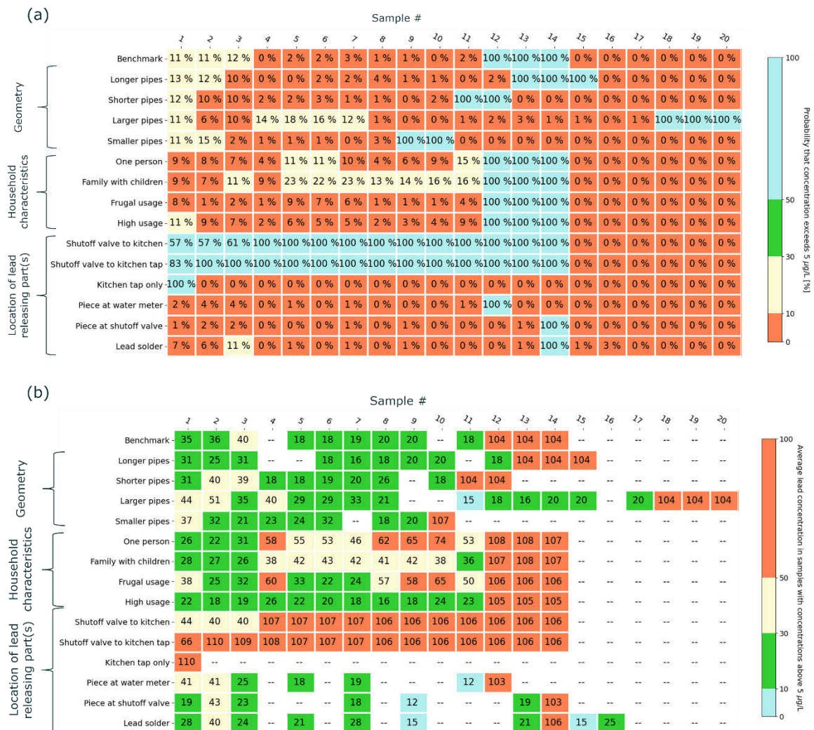
Figure 6: (a) Probability (in percentage) that a sample in a certain scenario contains dissolved lead with concentration above 5 µg/L. (b) Conditionally averaged lead concentrations in all samples wherein the dissolved lead concentration exceeds 5 µg/L.
