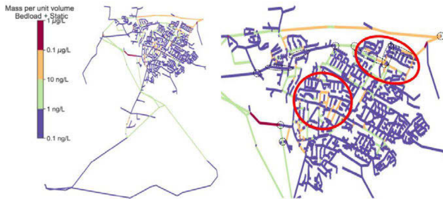
Figure 5. (a) Calculated sedimentation configuration for the reference scenario (RFS) of Castricum after 30 days, and (b) zoom-in of the same scenario. The encircled red areas show distribution pipe clusters of anomalously large sediment masses. The black dotted circles and ellipses show area where >300 mm transport mains connect to distribution pipes smaller than 300 mm.
