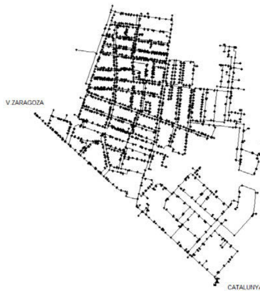
Figure 2. Hydraulic model of Benimaclet sector in Epanet [Source: ]
