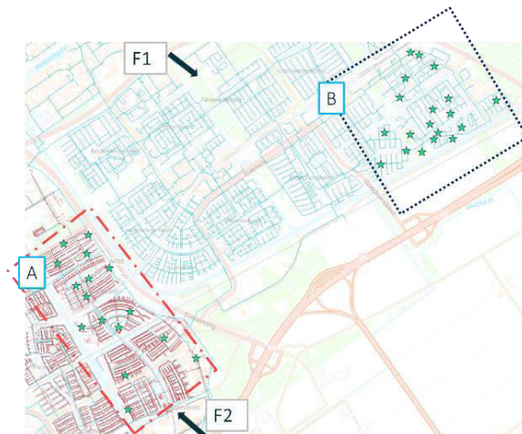
Figure 4 Almere DWDN in blue, and DHN in red. The measurement locations are indicated in green.
