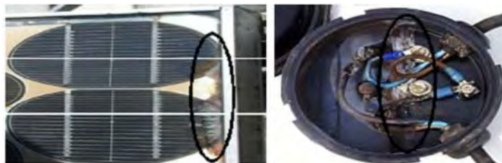
Figure 49. Corrosion of the a) Edge and b) Junction Box (81).
