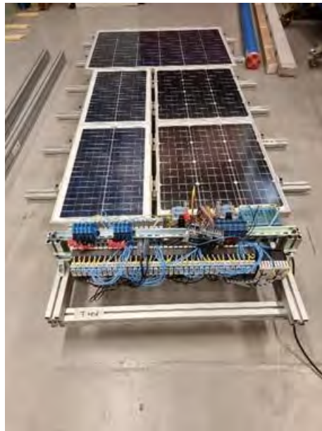
Figure 76. Complete PV System Simulator Assembly.
