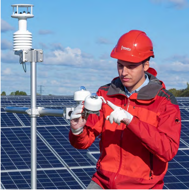
Figure 5 SR30-M2-D1 includes a digital tilt angle measurement, very practical for remote checks of instrument orientation. The image shows two SR30's in PV system monitoring, one measuring in Plane of Array (POA).
