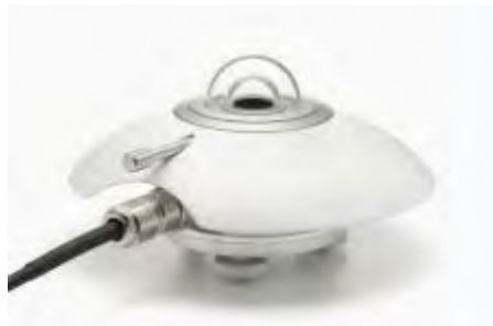
Figure 19. Irradiation Measurement: Pyranometer (46).
