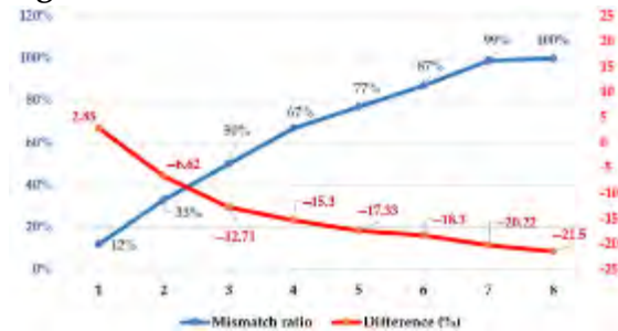
Figure 43. Chart of the Different Rates Compared to the Electrical Mismatch Ratio (79).
