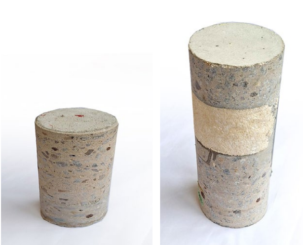
Figure 4 | Concrete sample cylinders of the GOMOS module. Single-layer 16cm thick on the left; triple-layer 30 cm thick on the right, credits: SUMMARY.
