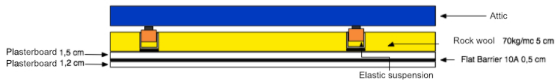
Figure 7 | Diagram of the floating ceiling.
