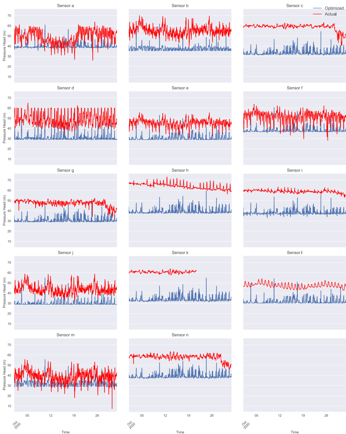
Figure 8. Comparison of optimized and actual pressure heads (m) at network junctions where pressure sensors are available. The optimization constraints at these junctions specify that pressures must be above 29 m (41 psi). The purpose of this plot is to illustrate how the levels of service in the form of pressure constraints are being applied and respected.
