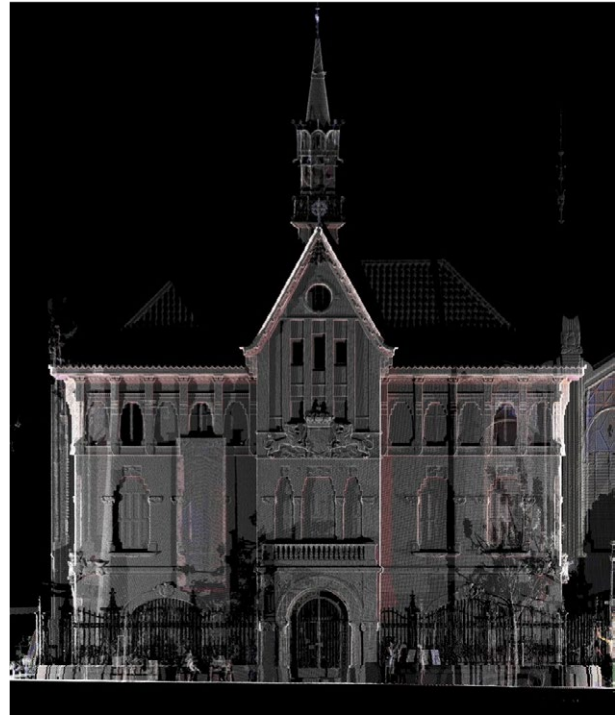
Fig. 9. Orthophoto of the main elevation of the point cloud
