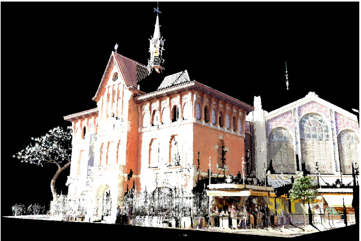
Fig. 8. Perspectives extracted from the point cloud
