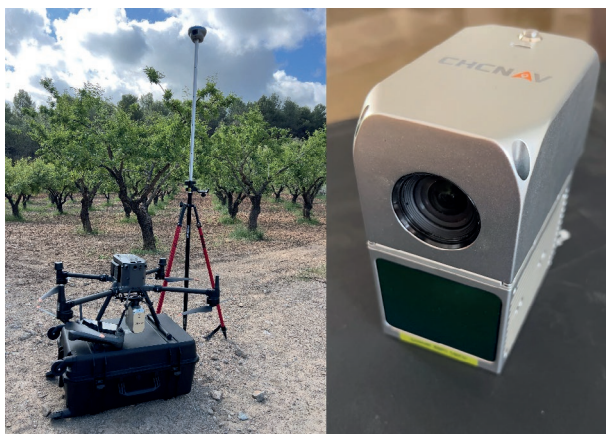
Fig. 4. DJI M350 RTK Equipment – AA450 LiDAR - i89 GNSS
