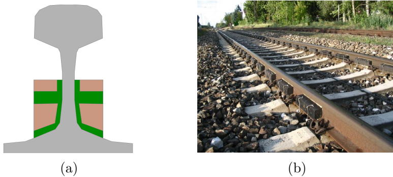
Fig. 2.11: (a) Rail tuned absorber (elastomers in green and steel masses in orange), adapted from [125]. (b) Dampers attached to the rails, extracted from [128].
