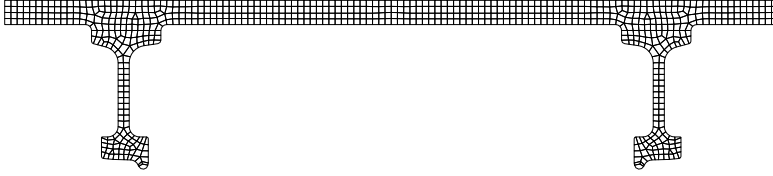
Fig. 2: FE mesh of the wheelset cross-section.
