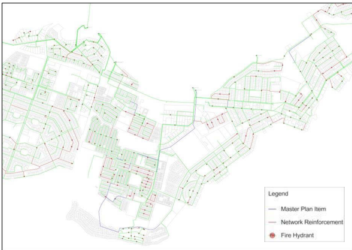
Figure 6. Test Case Network upgrades
