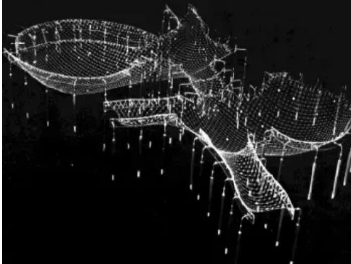
Figure 58 Picture showing hanging chain model used by Frei Otto for the Mannheim Multihalle 72
