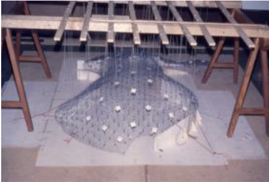
Figure 70 Picture showing the lifting positions model presented to the contractors 84
