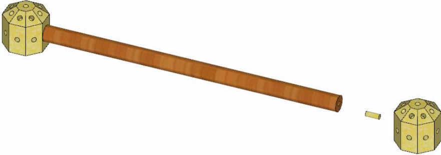
Figure 316 3D sketch showing the space frame base construction process – 1
