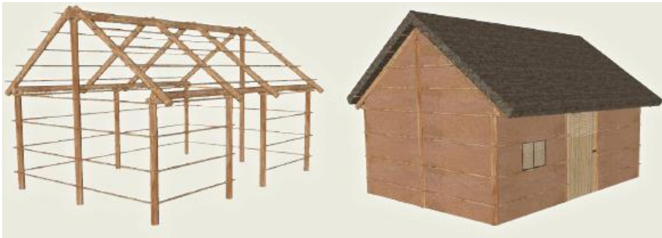
Figure 175 Picture showing the shelter unit with wooden structure, tarpaulin for flooring, corrugated iron sheets and thatch for roofing and adobe plastering for wall cladding 192
