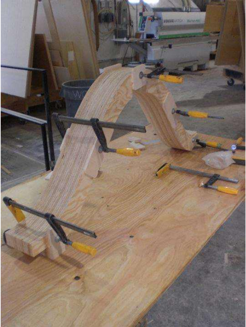
Figure 145 Picture showing the plywood clamped during the gluing process 162
