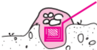
Figure 249 Sketch showing ground fixing by digging a trench, wrapping the sheets around timber and then covering them with earth and stones 268
