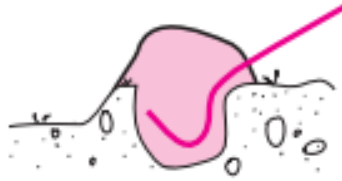
Figure 247 Sketch showing ground fixing by digging a trench and covering the sheet with earth 266
