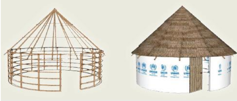
Figure 180 Picture showing the shelter unit with wooden structure, thatch for roofing and tarpaulin for wall cladding 197
