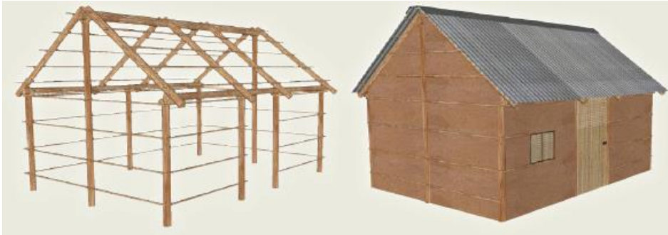
Figure 174 Picture showing the shelter unit with wooden structure, tarpaulin for flooring, corrugated iron sheets for roofing and mud cladding for wall cladding 191
