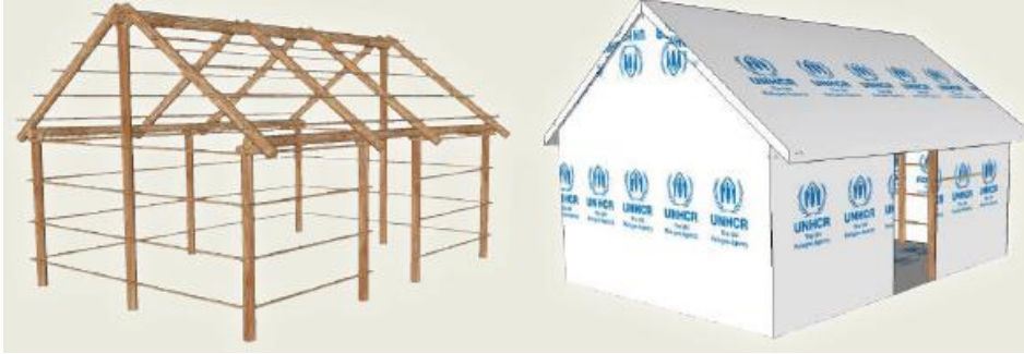
Figure 171 Picture showing the shelter unit with wooden structure and tarpaulin for the envelope 188
