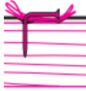
Figure 236 Sketch showing bended nail fixing through folded plastic sheet 255
