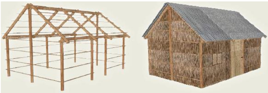
Figure 173 Picture showing the shelter unit with wooden structure, tarpaulin for flooring, corrugated iron sheets for roofing and thatch for wall cladding 190
