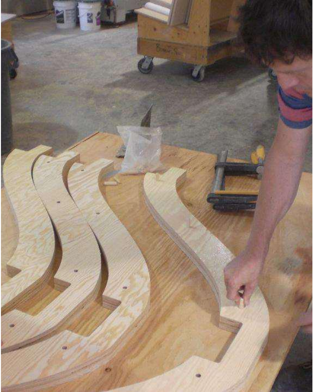
Figure 144 Picture showing the plywood laser cut pieces being joined together before the gluing process 161
