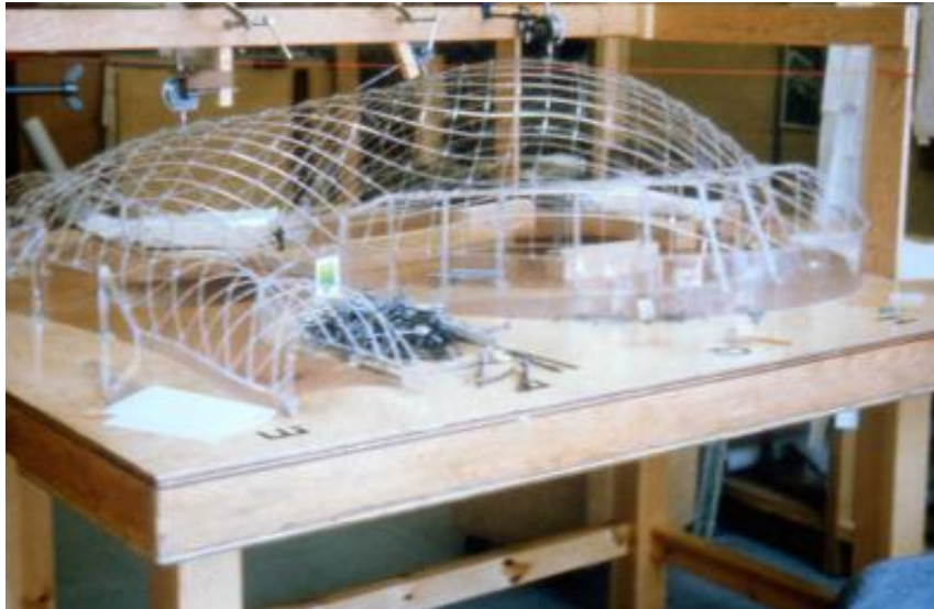
Figure 65 Mannheim Gridshell load testing model 79
