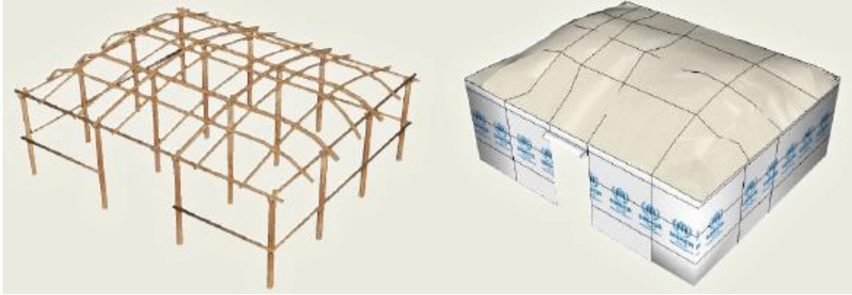
Figure 176 Picture showing the shelter unit with wooden structure and tarpaulin for the rest of the envelope 193
