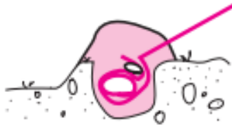
Figure 248 Sketch showing ground fixing by digging a trench, wrapping the sheets around rocks and then covering them with earth 267
