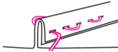
Figure 255 Sketch showing rope fixing by cutting a hole without or outside a reinforcement band 274
