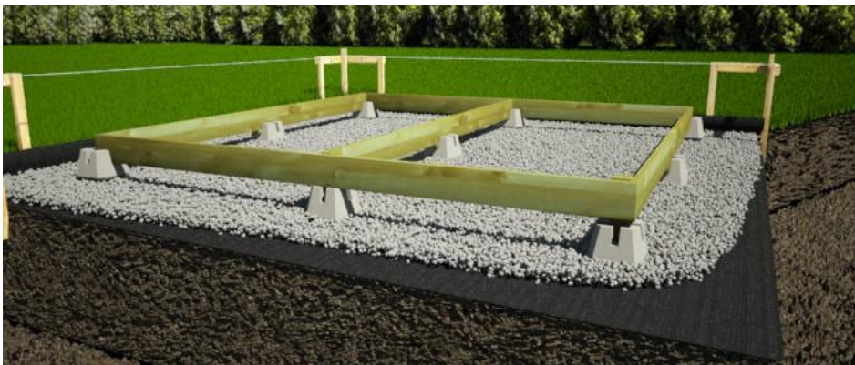
Figure 262 Sketch showing blocks with primary timber structure 281
