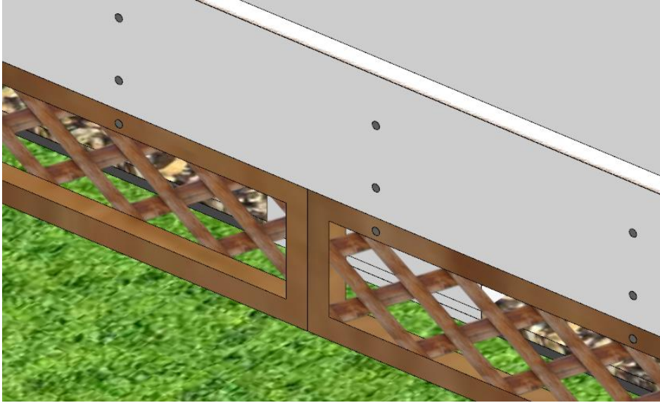
Figure 338 3D sketch showing the nailing patterns of the floor cover layer
