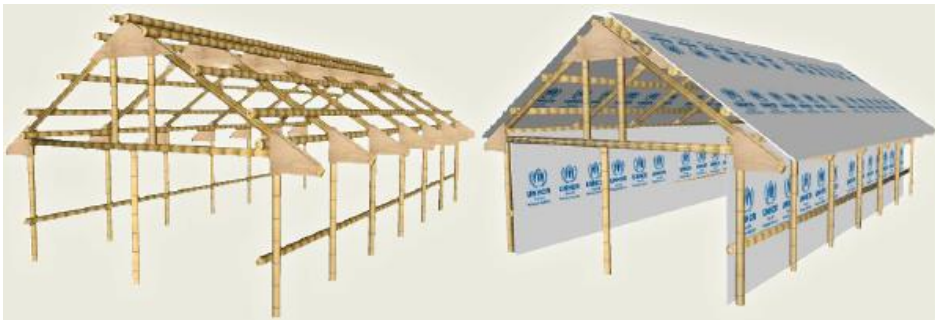
Figure 184 Picture showing the shelter unit with wooden structure and Tarpaulin for roofing and wall cladding 201
