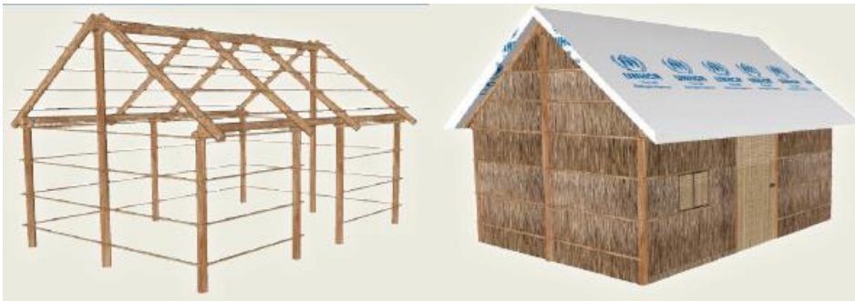
Figure 172 Picture showing the shelter unit with wooden structure, tarpaulin for roof and flooring and thatch for wall cladding 189
