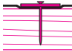
Figure 239 Sketch showing nailing through washers 258
